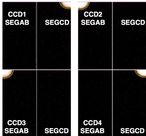
Figure 4: SXI image obtained during the FNC-N thermal vacuum test. Note that the images are given in the RAW coordinate. The left-bottom corners are (\text{RAWX}, \text{RAWY}) = (0, 0) .
