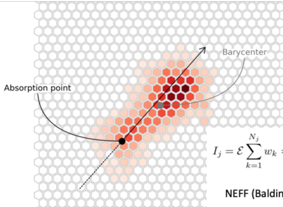
Pipeline processing computes moments of the electron track distribution to determine the photon absorption point and photoelectron initial direction.
